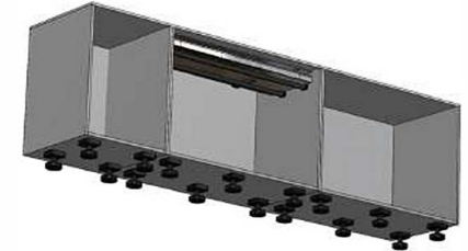
A3. Install the PITT Cooking Support bar set according to the PITT Cooking instruction manual.
