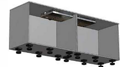
C1.2. Install the two PITT® cooking Units according to the PITT® cooking Installation and handling instructions.
